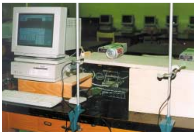
Fig. 1: A can rolls down the incline through a speed trap created by two lasers (background) and two laser switches (foreground). The first beam is at the top of the incline and the second is 50 cm away. The block at the top of the incline ensures that the cans always start at the same place.
